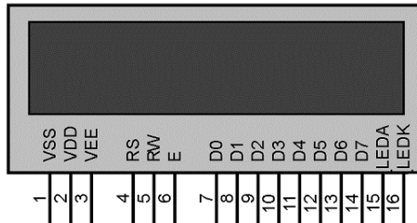
Fig. 2. Pins configuration of LCD 16×2
